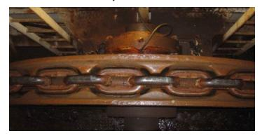
These chutes are lined with special materials to handle wear and tear and keep noise under control. Each chainwheel drive has a hydraulic disc brake to stop the ferry. There are over 1,000 sensors per ferry and staff carry out constant visual checks to ensure that any problem is flagged up as early as possible.
