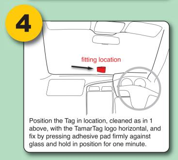
Certain vehicles are fitted with metallised or re-radiating windscreens, which can interfere with the electronic tolling communications. These screens can usually be identified by the blue/copper appearance of the glass. Generally such screen types have a window in the metallised area to allow Tags to communicate with toll equipment. If your vehicle is fitted with such a screen or are unsure whether it is so equipped, you must refer to your vehicle's manual and/or service agent.
